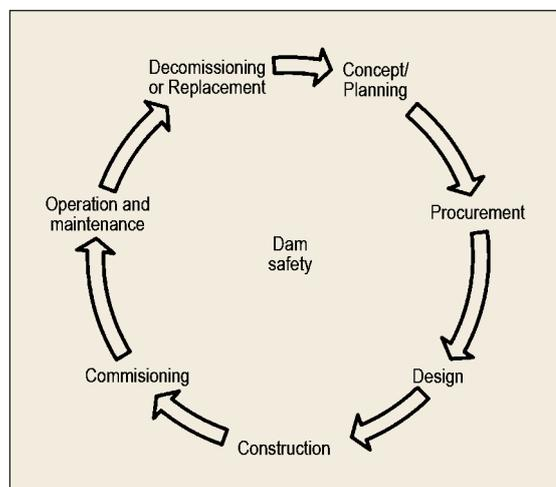
Fig. 1. Dam safety requirements over the lifecycle of a dam (adapted from ICOLD Bulletin 154 [In press<sup>3</sup>]).
