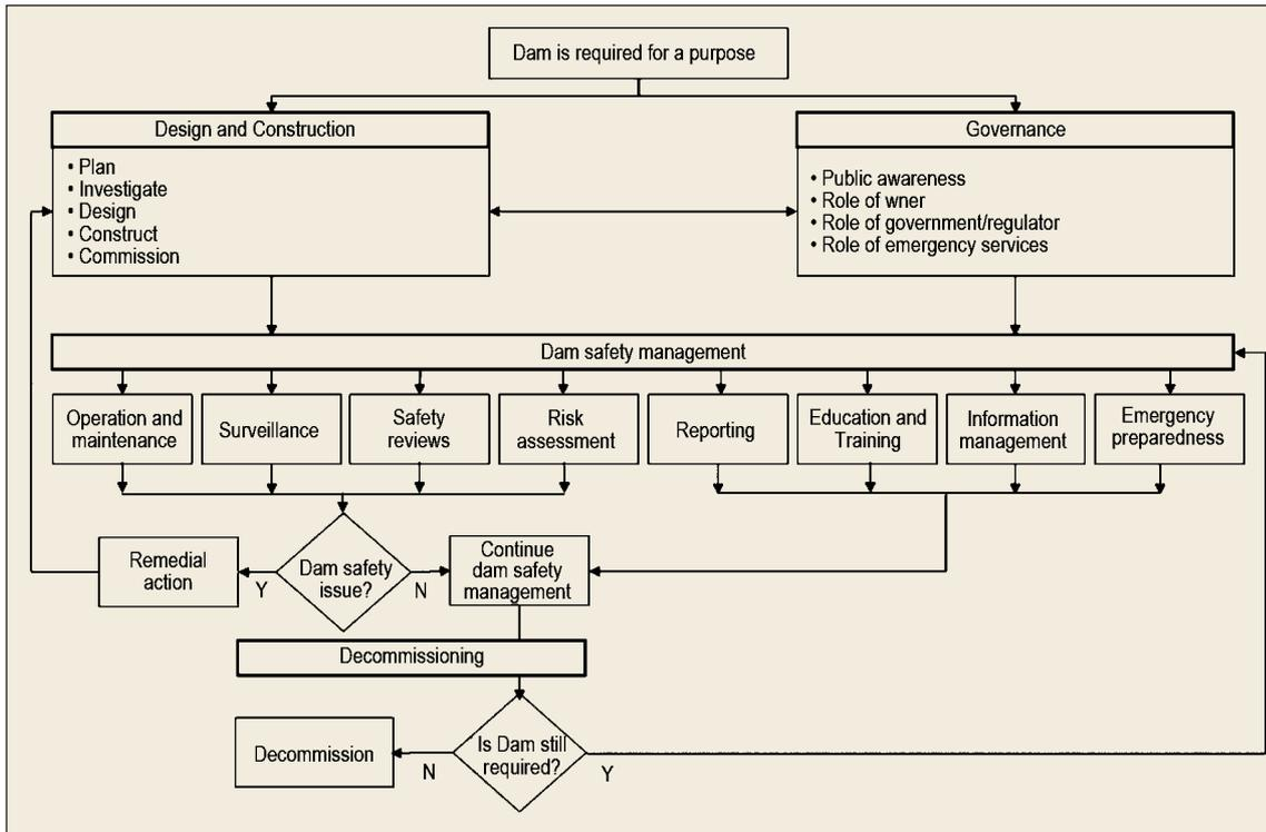
Fig. 2. Elements of a dam safety management system [adapted from ANCOLD, 2003<sup>10</sup>].
